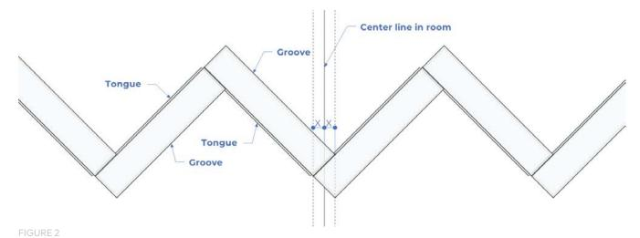
Determine the center line and starting position as illustrated in Figure 2.
